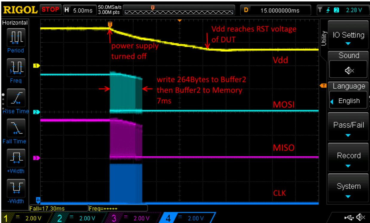
Figure 3. Oscilloscope Output of Experiment 1
