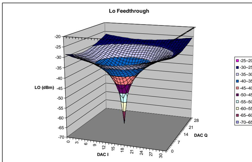
*Measurement results from a production sample showing feed-through contours*
