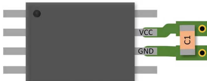
Figure 8. Placement of Decoupling Capacitor on an Adesto SOIC Device with Adjacent VCC/GND Pins
